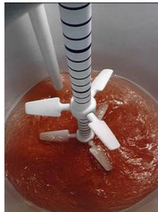
Figure 1.2.D. Glass-lined agitator shaft with two sets of impellers. A baffle can be seen to the upper left of the agitator shaft.
