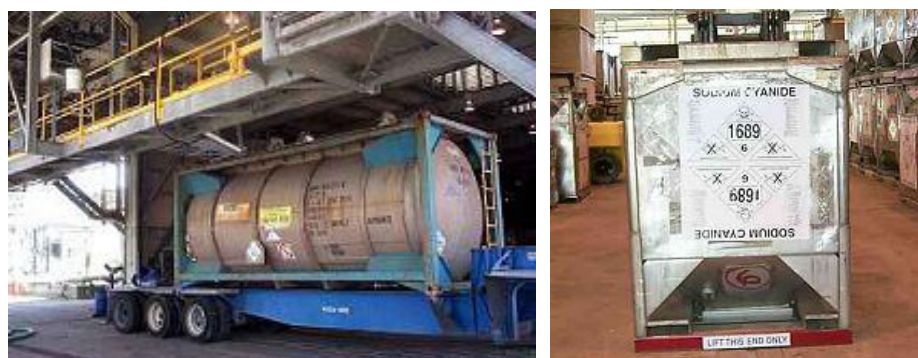
Figure 45.C. Larger bulk containers for NaCN. Left: ISO container; Right: Returnable steel bin.
