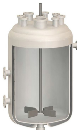
Figure 1.1.A. Cut-away view of a chemical reaction vessel with a cooling jacket, showing agitator shaft and blades. The connections on the sides of the vessel allow for cooling fluid to circulate between the inner and outer vessel walls.
