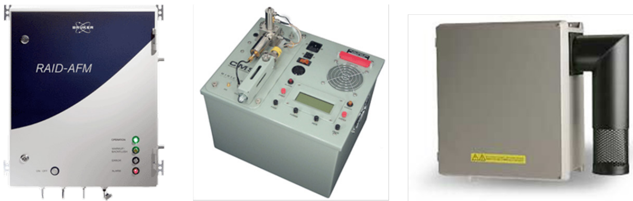
Figure II.A. Toxic gas monitoring systems for CW agents. Left: Ion mobility spectroscopy -based system; Centre: Gas chromatography -based system (different detector options available); Right: Surface acoustic wave spectroscopy -based system.
