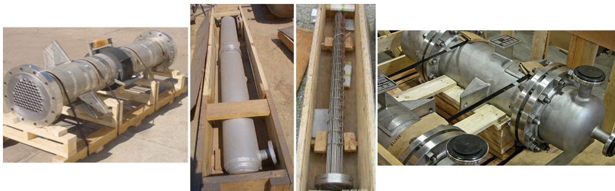
Figure 3.F. Packaging for shell and tube heat exchangers, condensers, and tube bundles. For final shipment, the heat exchanger on the left would probably have its ends sealed to prevent debris from entering the tube bundle. The units on the far right are condensers, the left and centre left units are heat exchangers, and the centre right image is of a tube bundle.”
