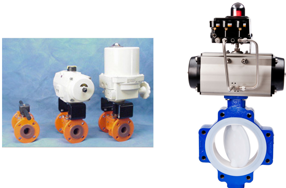
Figure 6.A. Fluoropolymer valves in a variety of designs. Left: PFA-lined plug valves with different actuation mechanisms (manual, pneumatic, and electrical); Right: 6 inch (DN150) PFA-lined butterfly valve with pneumatic actuator, indicator, and limit switch enclosure.
