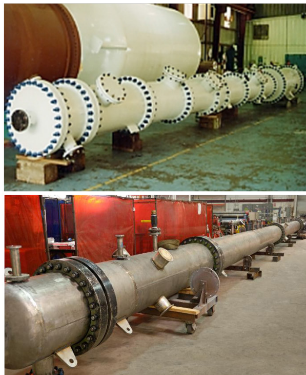
Figure 4.A. Distillation columns. Left: Simplified schematic of a distillation column showing packings, trays, and selected column internals. Components are not to scale. Right: Complete distillation columns lying on their sides (with ports covered).
