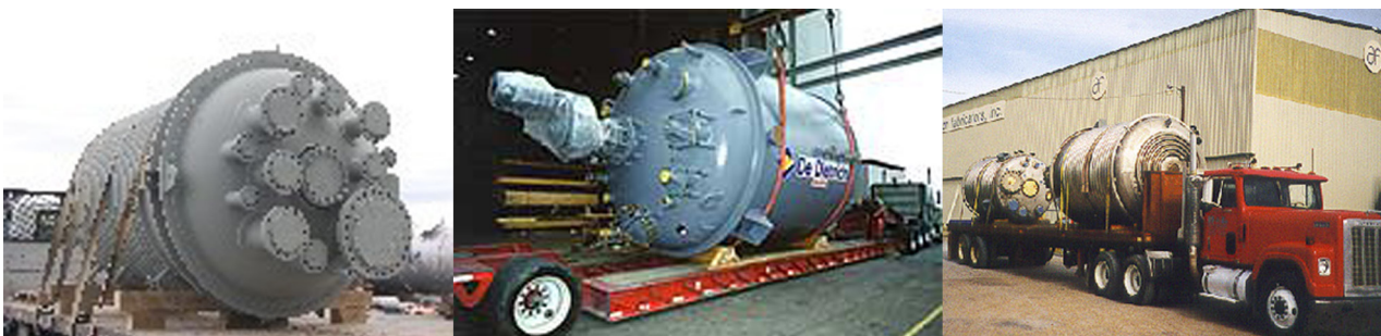
Figure 1.1.F. Reaction vessels with sealed ports strapped to trailers for shipment. The image on the left is a Zirconium 702-clad reactor. Note: the volume and – by extension – the control status of these reaction vessels is unknown.
