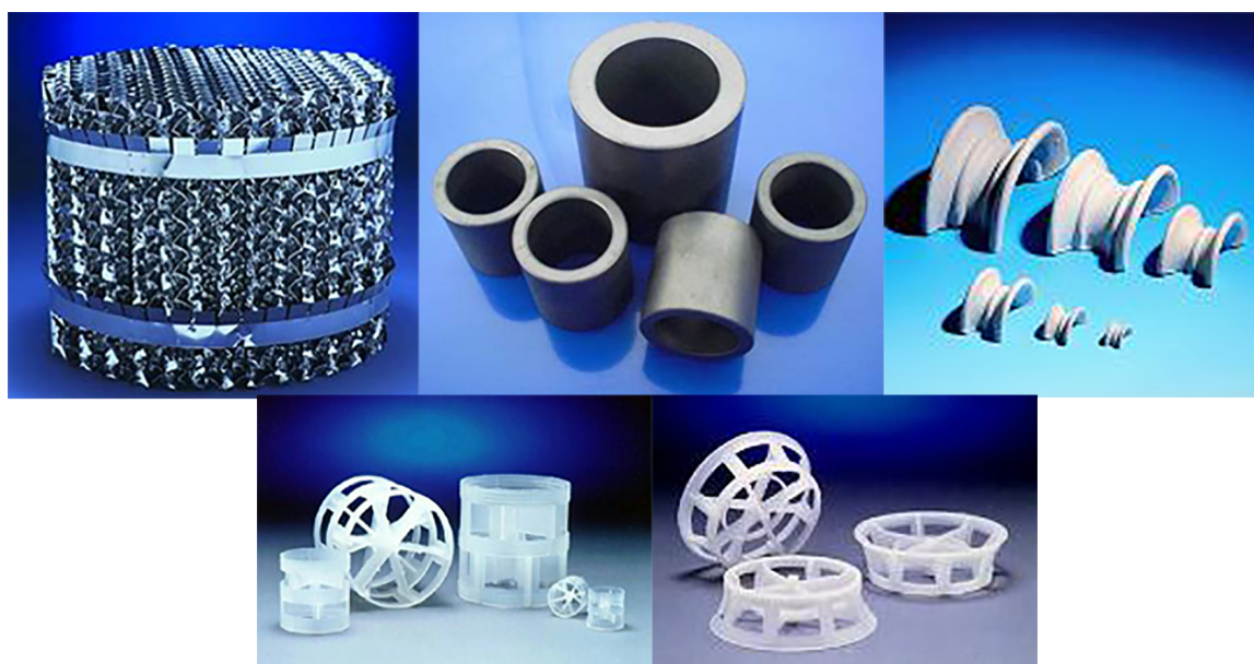
Figure 4.C. Structured and random packings for columns. Top left: Corrugated metal structured packing; Top centre: Carbon Raschig rings; Top right: Ceramic Torus Saddles; Bottom left: Plastic rings; Bottom right: Plastic low profile rings.
