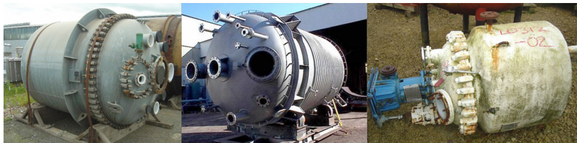
Figure 1.1.C. Left: 6000 litre glass-lined vessel; Centre: Hastelloy C-276 half-pipe reactor; Right: 450 litre fluoropolymer-lined reactor.
