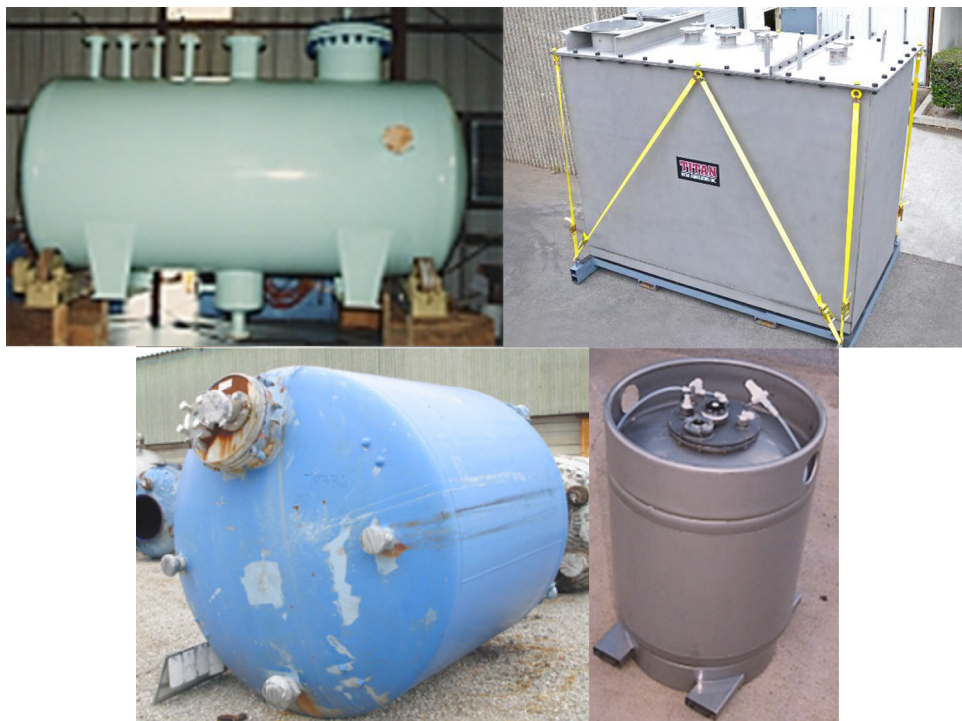
Figure 2.A. Simple storage tanks and containers. Top left: Glass-lined horizontal tank ; Top right: Zirconium alloy storage tank ; Bottom left: Glass-lined vertical tank ; Bottom right: Fluoropolymer-lined IBC .
