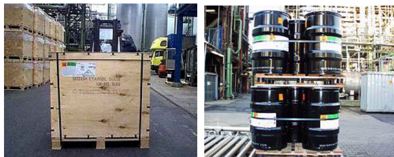
Figure 45.B. Bulk containers for NaCN. Left: Wooden box with inner bag; Right: Palletized steel drums.
