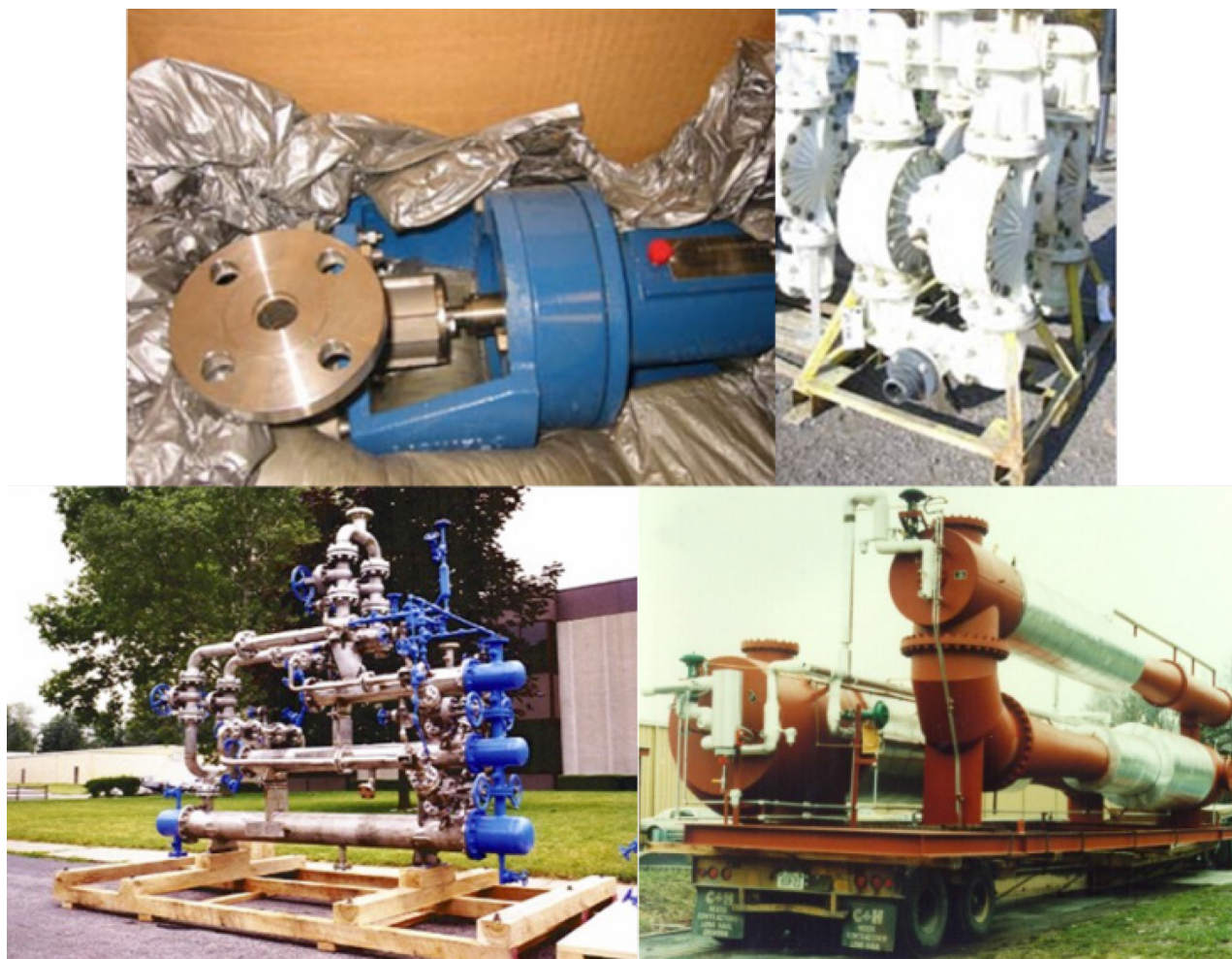
Figure 8.F. Pumps ready for shipment. Top left: Centrifugal pump head in a box with padding; Top right: Diaphragm pump strapped to a pallet; Bottom left: Multi-stage ejector pump system on a pallet; Bottom right: Ejectors on a flat-bed trailer.
