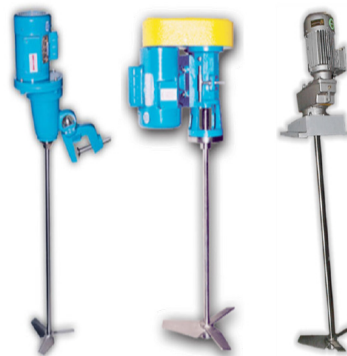
Figure 1.2.A. Complete agitators with a variety of motor and mounting options. Left: Gear drive motor with C-clamp mount; Centre: Belt drive motor with flanged mount; Right: Gear drive motor with angle riser and plate mount.
