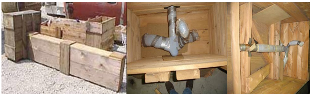
Figure 1.2.F. Crated agitator shaft-impeller units. Left: Crate with larger box to accommodate impeller. Centre: Protectively-wrapped glass-lined impeller; Right: View of wrapped and shaft in a one-size crate.
