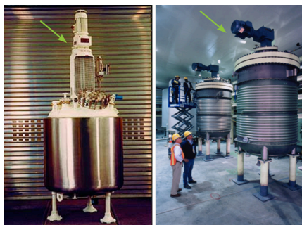
Figure 1.1.B. Chemical reaction vessel designs with agitators. The green arrows are pointing to the agitator motors protruding from the tops of the vessels. Left: 500 litre glass-lined reactor with welded top head and smooth sides; Right: Reactors with visible temperature control coils and bolted top heads.
